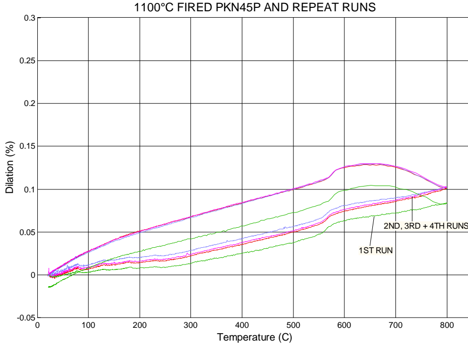
Figure 38: Four Runs of 1100°C Fired PKN45P
