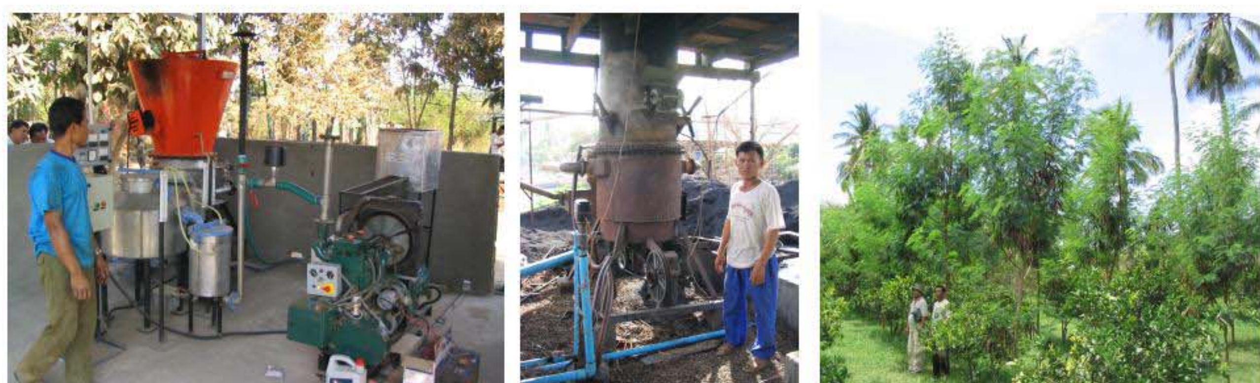
Figure 4. There are currently two biomass gasification power plant operating and supplying electricity to total about 500 households. Far Left; 9 kW system operated by village energy cooperative. Middle; Gasifier invented by local engineer, operated by duel fuel (with diesel). Near Left; One year old Leucaena leucocephala planted with orange, the branches are used for fuel for power generation.
