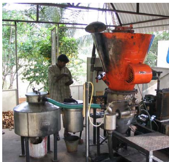
Figure 3. The 9 kW gasifier system installed for Odanthurai Panchayat water supply system in Tamil Nadu State.
