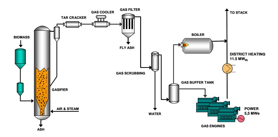
Figure: Simplified flow sheet of the BGGE plant in Skive.
