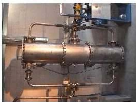
Figure 18. Reverse Flow Tar Converter.
