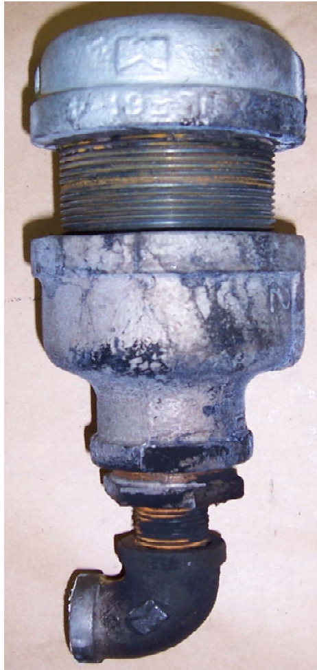
Figure 6: Final Boiler Design
