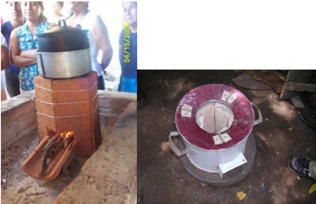
Six of these trapezoidal bricks will make the combustion chamber of a Rocket stove.
