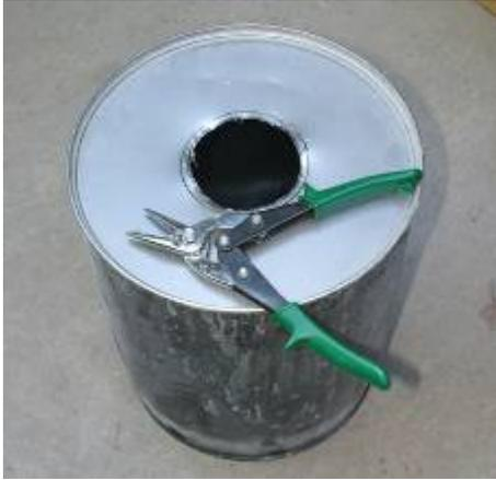
Using tin snips, cut out the inner circle.
