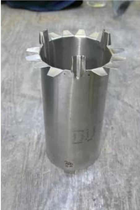
The tabs at the upper end of the riser piece are folded down to create the structures that will hold the riser onto the top of the stove body (can). The three crimped tabs, which will serve as the pot supports, are bent outward for additional mechanical strength.
