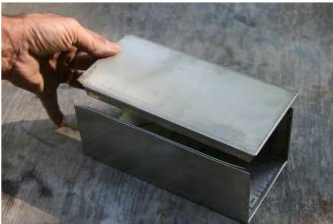
The fitting together of the top and bottom pieces of the fuel magazine.
