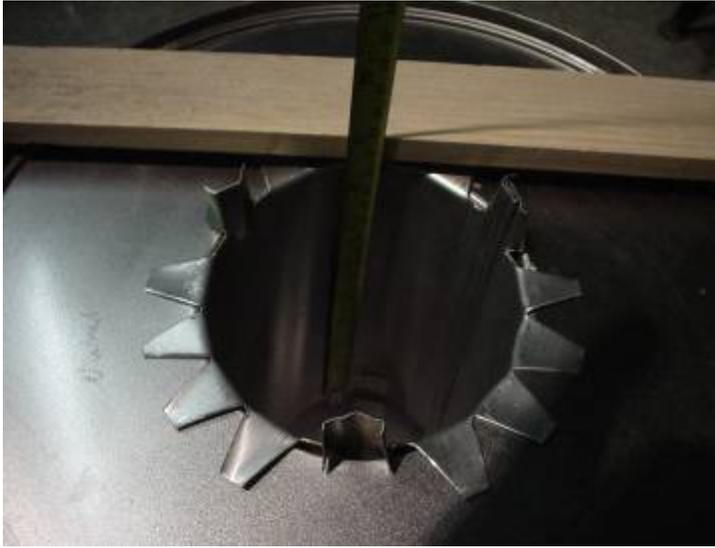
Using a straight edge across the top rim of the can, measure vertically to the bottom of the riser tube.
