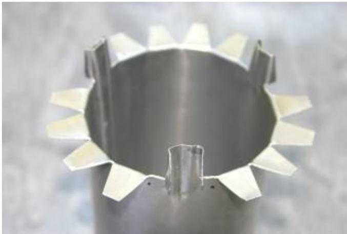
Detail of the cuts and folds on the top end of the riser.
