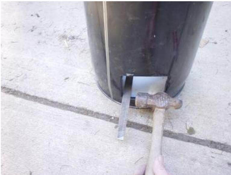
Since the hammer edge is round, but we need square corners to accommodate the fuel magazine, I used a hard, rectangular object to form them. For example, pound on the side of a heavy metal file set against the corner to square-up the bend.
