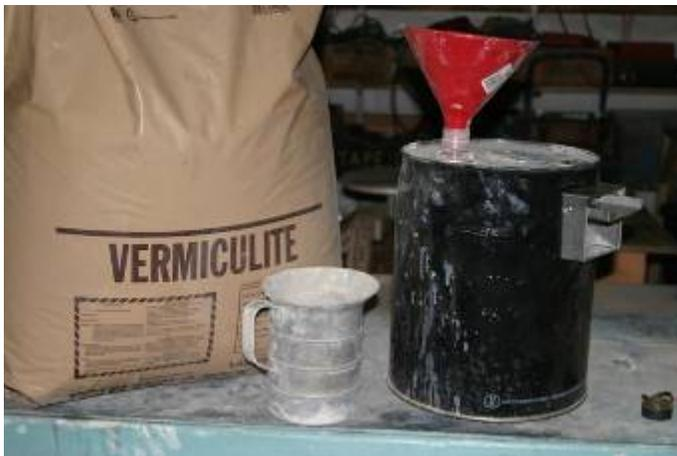
Using the spout on what is now the bottom of the can, fill the stove body with insulation. Wood ash is an excellent insulation material. I used vermiculite.
