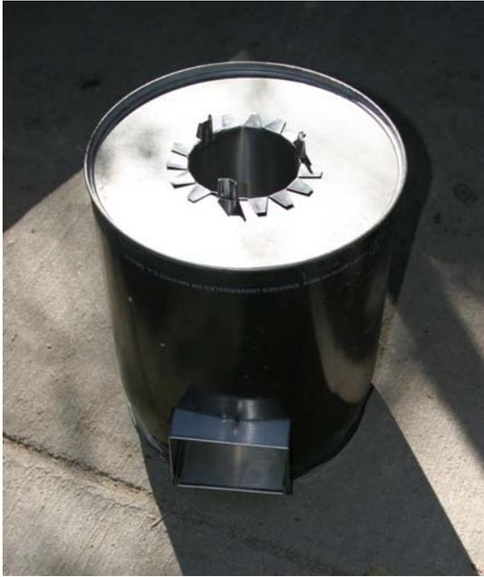
The combustion chamber is now in place within the stove body.
