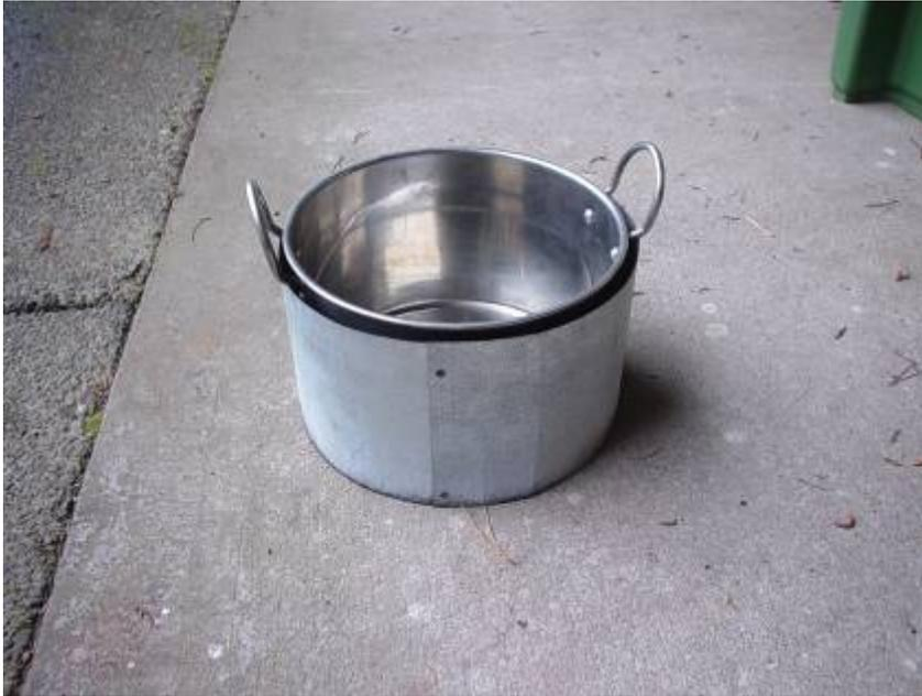
Assemble the pot-skirt by measuring and cutting thin galvanized sheet into a properly sized strip, and fastening with three pop rivets. It is important to achieve the proper "Gap D" between the pot wall and the skirt so as to maintain the same cross-sectional area throughout the stove, from magazine opening, through the riser, and around the pot.
