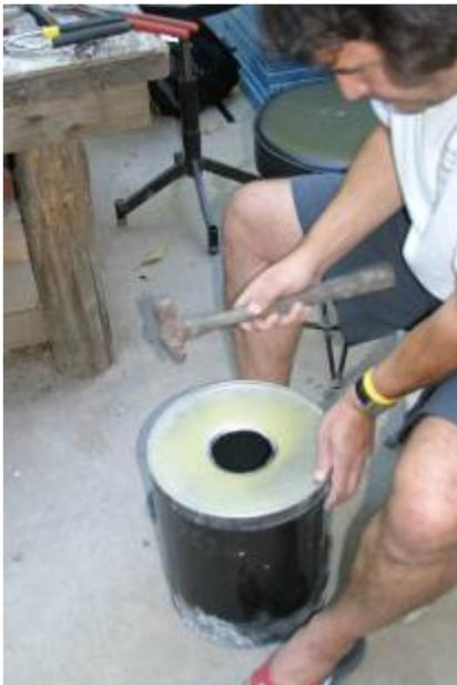
Bending down the annulus for the riser placement, using the ball-end of the ball-peen hammer.
