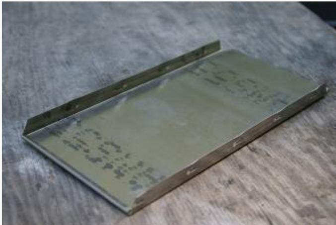
The edge of the bottom piece has been crimped to snap into the fold of the larger piece.
